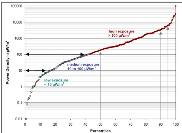
**Fig. 5. Exposure levels to HF radiation of a GSM cellular tower base station** (Haumann and Muzenberg, 2011)
