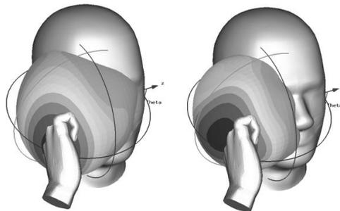
**Fig. 1 GSM Band Antenna Radiation Pattern from a Cell Phone
