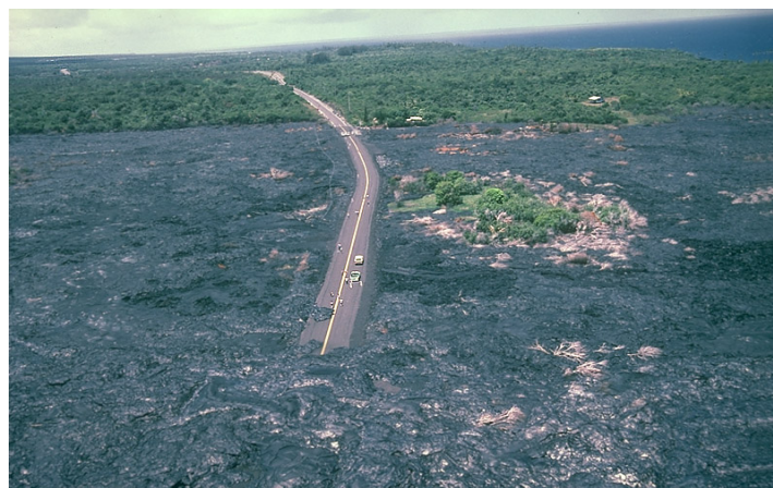
Fig. no 5. Lava blocking the highway No 130 on the South-Western coast of the Hawaii Island, the USA on February 23, 1990. During multiple eruptions of Kilou volcano in the period of 1983-1998, lava flows blocked nearly 13 km of the highway to the depth of about 25 m. The total buried territory was 99.7 km 2 . Photo Credit: J. D. Griggs, Hawaiian Volcano Observatory, U.S. Geological Survey, June 6, 1987
