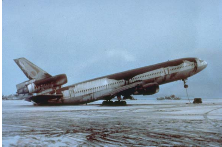
Fig. no 1. Structural damage of the CD-10 airplane at U.S. Naval Air Station in the Philippines. Photo Credit: R.L.Rieger, made on June 17, 1991.
